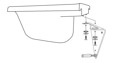
**4. Attach the P-Trap** (not supplied) to the #1733 Basket Strainer. Connect the #550 Fixture to the hot and cold supply lines. Apply a bead of silicone to the back edge of the bowl to seal it to the wall.
