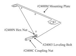
3. Mount the Model #4000 Shampoo Bowl. Remove the mounting bolts, washers and lockwashers from the back of the bowl. Set the bowl in place on the mounting plate and fasten using the bolts, washers and lockwashers. Insure the bolts are tightened securely and that the bowl is flush with the wall or cabinet. Level the bowl by adjusting the 2400C Coupling Nut.
