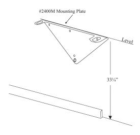
**2. Leveling Bolt Installation.** Install the #24003 Leveling Bolt all the way into the #2400M Mounting Plate and tighten the #2400N Hex nut to secure. Thread the #2400C Coupling Nut all the way on to the opposite end of the Leveling Bolt.
