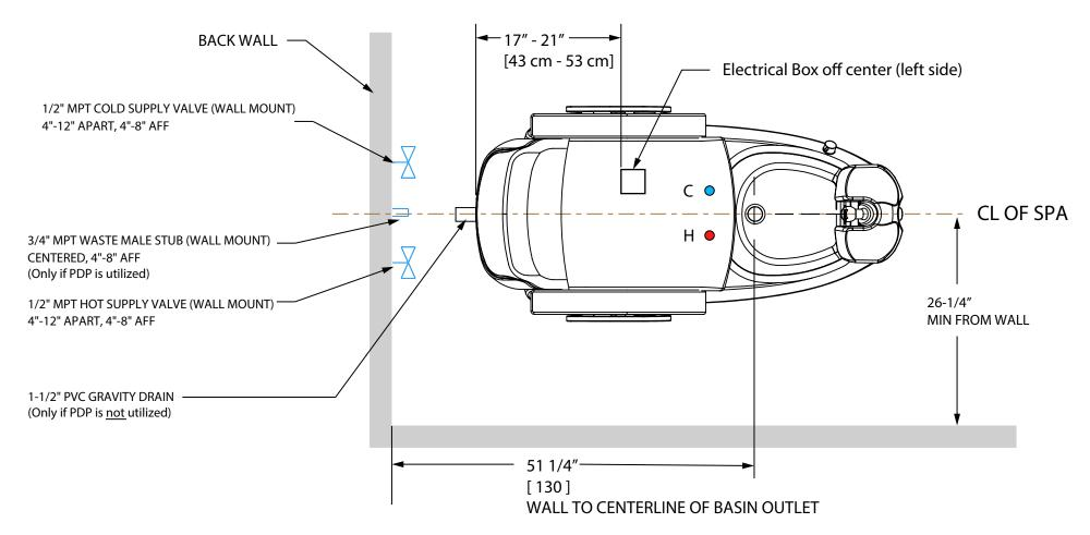
•Electrical Requirements: One (1) dedicated 15 amp, GFCI protected wall outlet/circuit per unit located within two (2) feet of the rear of the Pedicure Chair. (Actual draw is 5 amps) Each Pedicure Chair will be supplied with a standard 40" grounded power cord. If utilizing an in-floor electrical box (4" round), position box underneath spa approximately 17"-21" (43 cm - 53 cm) off centerline (left side) from back edge of fiberglass base.
