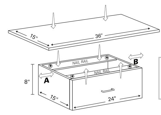
Tip: On the back of both pieces place a mark IN THE CENTER of each unit. Align the two marks together and the station should be centered.
