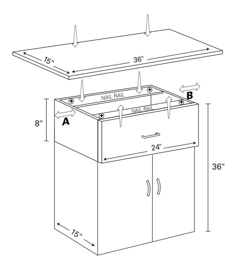
Tip: On the back of both pieces place a mark IN THE CENTER of each unit. Align the two marks together and the station should be centered.
