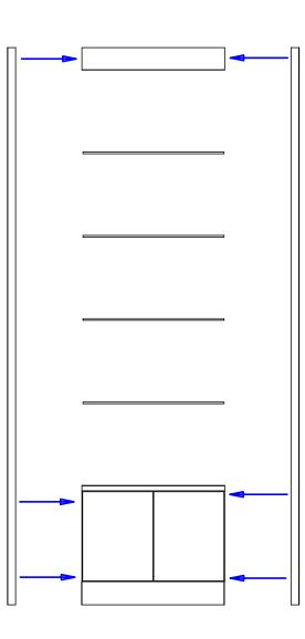
This item is attached to the wall with wood screws. 3" wood screws and decorative washers are provided for wood framed walls. Fasteners for other wall types are to be obtained locally. Screw through the back panel in locations which will be inconspicuous after installation. Suggested locations include: under shelves, behind drawers, and locations hidden by products or supplies.
