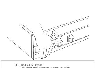
Pull the drawer fully open so levers are visible.
