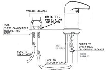
ENGLISH: Arrows on the vacuum breaker indicate directional flow of water. Device will leak and not work properly if installed with water flow reversed.
