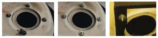
Place washer and nut on each insert and tighten to pull inserts tight to hold Remove nut, but leave washer on each insert.
