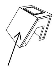
Shuttle Chases Are Used To Connect Adjuacent Backwash Shuttles, Hide The Connected Plumbing, & Maintain The Proper 32" Centers For The Chairs & Shampoo Bowls
