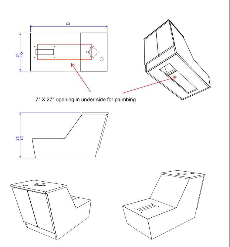
Backwash unit must be anchored to floor using either wood screws or concrete anchors depending on your floor type. All plumbing should be done by a licensed plumber in accordance with local code
